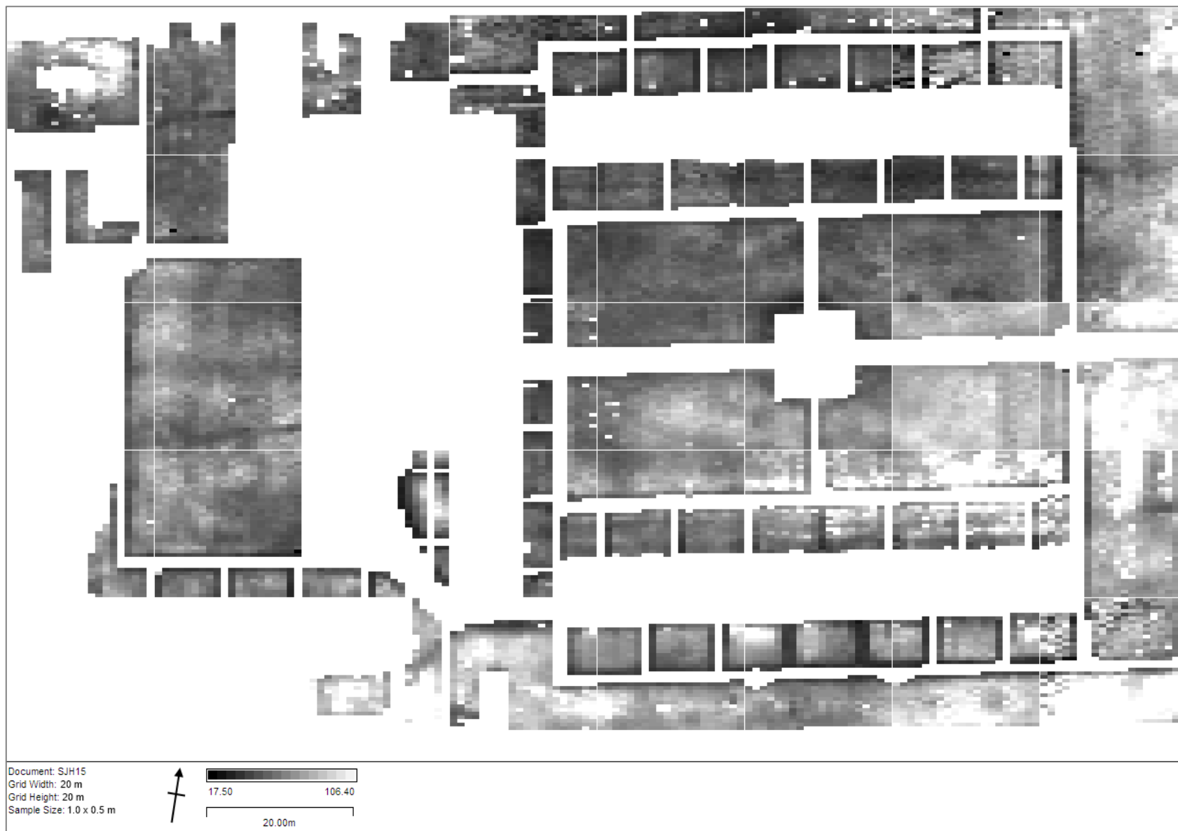
Figure 11. 'Raw' unprocessed resistance output. Copyright © 2015 Fishergate Fulford and Heslington Local History Society.
